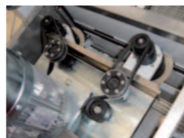
Mandrini spigolatori Supersonic Supersonic chamfering spindles
