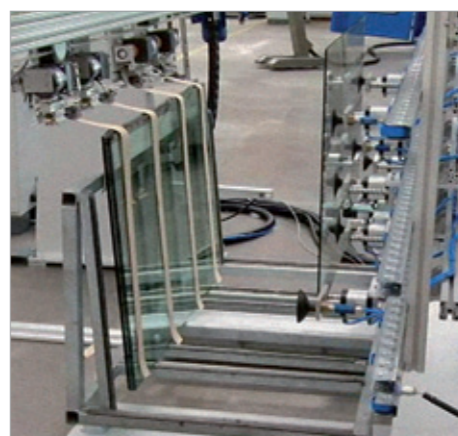
Automatic paper-spreading systems
